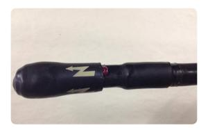
Note: As the cap shrinks it may begin to slide off. An insulated core wedge can be used to hold it in position.
