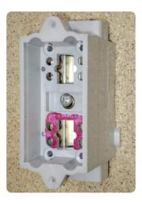
• The blanking plugs in the fuse carrier and neutral earth block are removed by inserting a 3mm insulated Allen key tool into the appropriate hole below the terminal screws.
