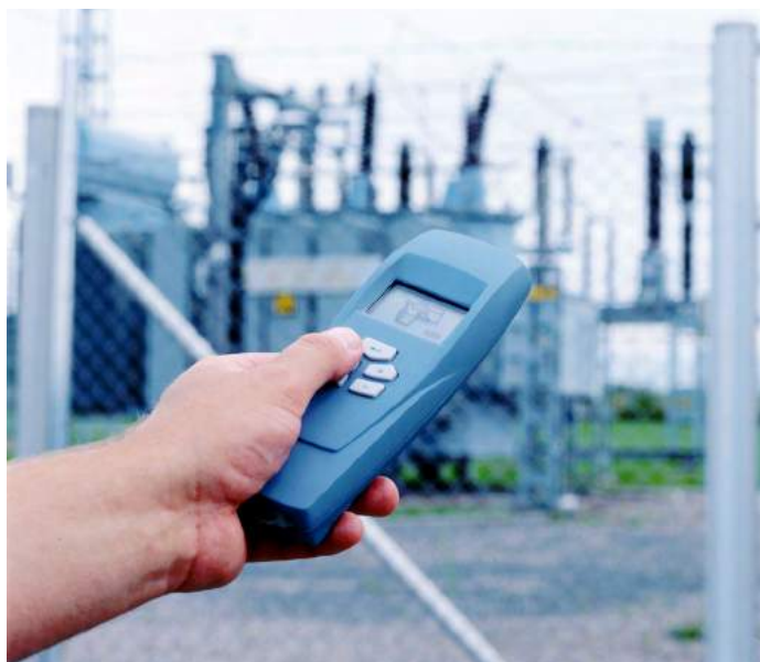
Remote reading with EXCOUNT-II
