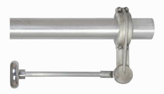
The machined clamp is supplied in two halves that are bolted together around the busbar using the supplied fasteners. A 38mm diameter spigot and corona shield, common to all spigot clamps and busbar sizes, is then bolted onto the clamp.
