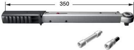
730R Torque wrench for bolt connectors, bolt cable lugs, overhead line clamps, etc. Supplied with 7 mm socket head, extension arm and 8 mm internal hexagon head. Torque range 6–50 Nm.
