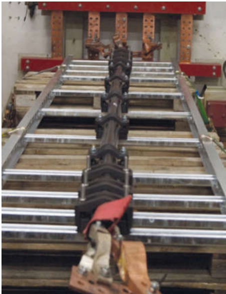
id-Technik Cable Clamps for trefoil formation before the test
