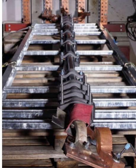
Cable Clamps for trefoil formation after the 1 st test
