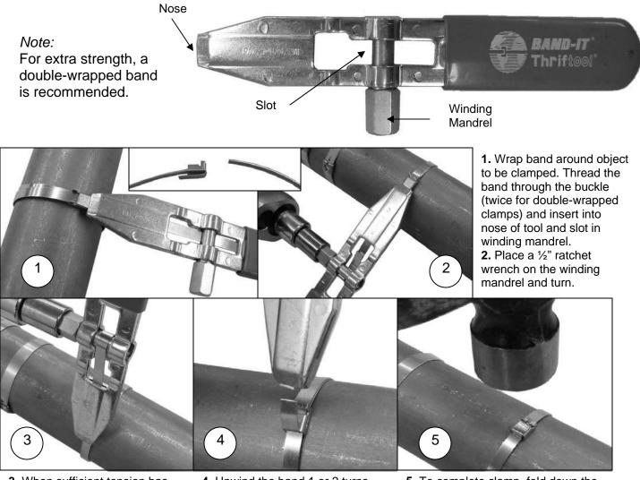
**3.** When sufficient tension has been applied, rotate the Thriftool<sup>®</sup> over the buckle.
