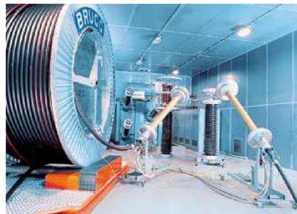
Brugg Cables' modern, fully screened test room for AC voltages up to 600 kV
