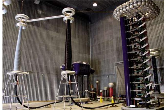
Prequalification test of 550 kV equipment
