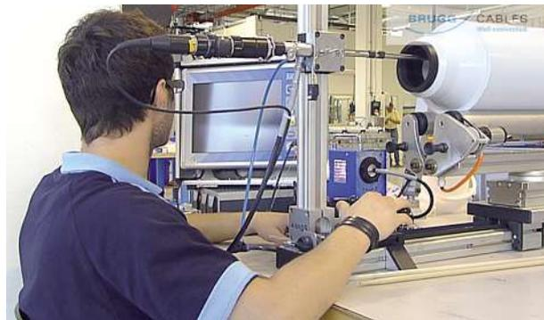
Single control of the surface of a SiR slip-on joint body after production
