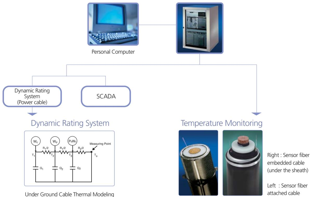
Thermal models and real-time temperature measurement can provide dynamic rating system. And this system allows qualification of actual cable capacity, cable conditions and environmental parameters critical to the stability and longevity of the cable system.
