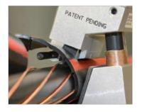
Recessed blade increases safety & is easily replaced.
