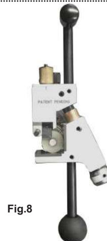
XLPE cable - remove semi-con first
