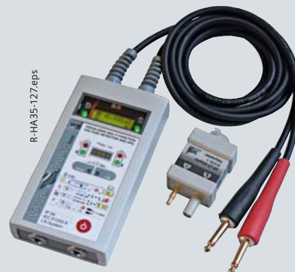
Phase comparison test unit make Hachmann, type VisualPhase LCD as combined test unit (HR and LRM) for: – Voltage detection with measured-value indication – Interface test – Low voltage detection – Documentable repeat test – Phase comparison with LED signal and measured-value indication – Phase angle from -180^\circ to +180^\circ – Phase sequence evaluation – Frequency quality – Complete self-test
