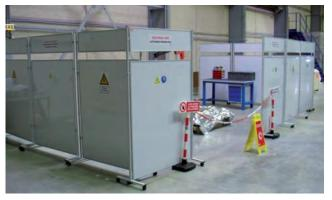
Modular panels easily transportable on a structure with casters and joints.
