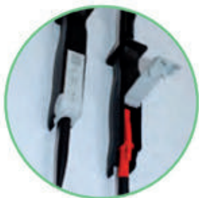
Hatch for storage of test probe.
