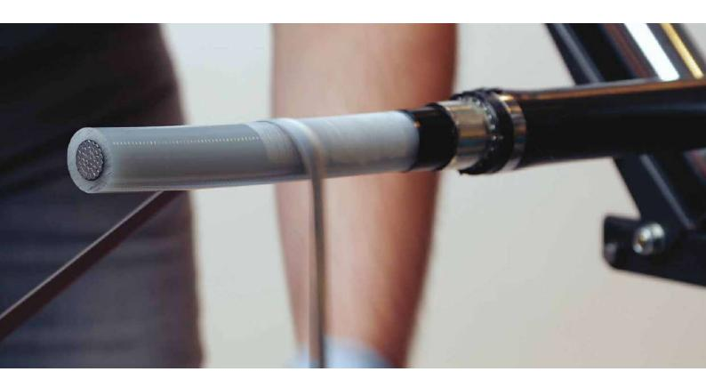
The insulation thickness is defined by the rated voltage of the cable. Cross-linked polyethylene (XLPE) and ethylene propylene rubber (EPR) are common insulation materials.
