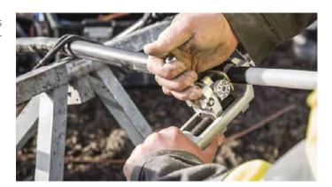
Ensto ST259 is an outer sheath spreading wedge that is also used to help open or remove the outer sheath of single and three-core cables of different constructions.
