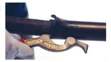
Ensto ST310 is for fastening metallic cable ties on the cable's outer sheath. With the metallic ties, the grounding grater makes an earthing contact to the aluminum laminate screen. The tool does the tightening and cutting of the exceeding tie.
