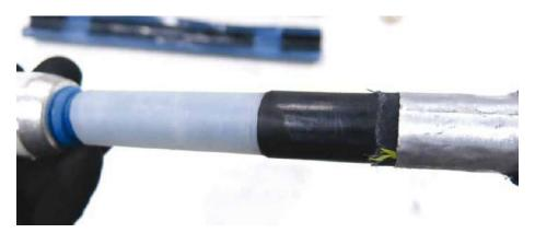
Grinding the insulation screen This cause conductive particles to spread all over the insulation, causing partial discharges.
