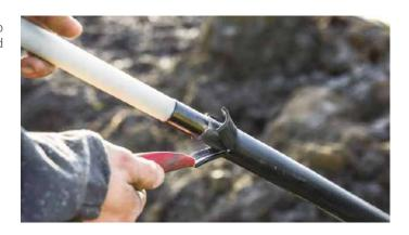
Ensto ST286 is used to spread the outer sheath and/or aluminum laminate. It does not harm the aluminum laminate or semi-conductive layer during spreading.
