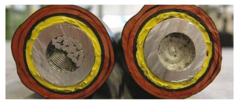
**Tubes shrank asymmetrically** Flame must be in constant movement and applied symmetrically all around the heat-shrink tubes.
