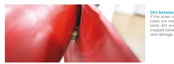
Dirt between tubes If the outer sheath is not clean or the tubes are not cleaned after shrinking, sand, dirt and/or small stones can be trapped between tubes and cause se-
