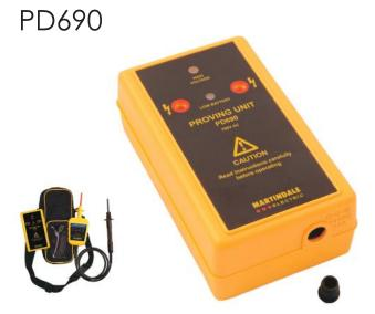
The PD690 proving device produces 700V AC/DC to enable voltage indicators and other devices with ranges up to 700V to be checked. It is a portable, battery powered proving unit with the option of being driven from a 12V supply via a car or mains power supply. The kit is supplied with a combination carry case for both VI and PD products.
