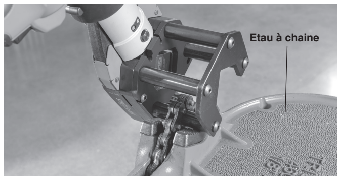
Figure 5 – Strut Shear Head Mounted in Chain Vise
