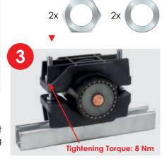
Alternating, tighten nuts with an appropriate torque wrench. Do not use self-securing/self-locking nuts, this prohibits a defined tightening torque.
