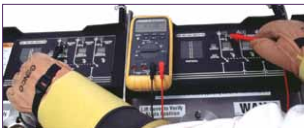
Figure 7. Measuring phase-to-phase voltage—Phase 1 to Phase 1.
