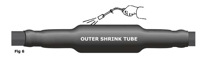
6. Clean and abrade the outer cable sheath before positioning the outer shrink tube centrally over the joint. Shrink from the centre to one end at a time. Keep the flame moving all around the tube to ensure an even wall thickness and good adhesive flow.
