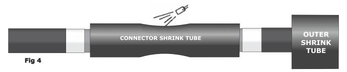
4. Centralise the connector insulation tube and with a suitable heat source, shrink from the centre to one end at a time all around the tube until fully recovered as in Fig 4.
