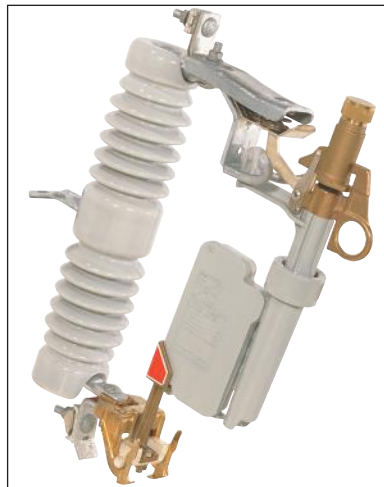
Figure 5. Catalog number 98072-D rated for 15-kV, 125-kV BIL systems. Includes extension adapter to allow 15-kV Fault Tamer Fuse Limiter components to be installed in 25-kV mounting.
