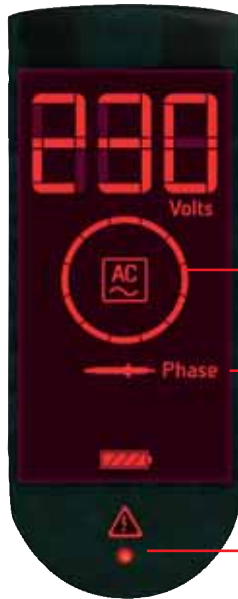
Example of detecting 230 V AC, displayed in RED .
