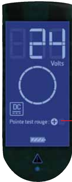
Example of 24 V DC detection, display is BLUE because < 50 V.
