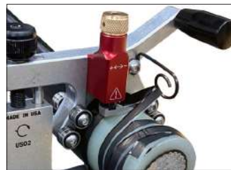
Winding loop keeps semi-con strip from getting in the way
