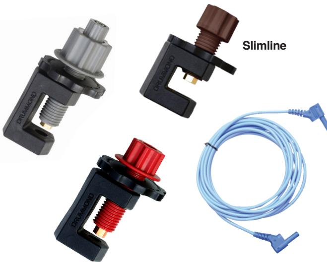
Drummond G-Clamps simplify bus bar connections with a clamp-on design. Ensuring a safe and reliable connection through a standard 4mm socket, the fluted head of the moulded screw include a 4mm shrouded socket. The connection is suitable for up to 10A continuous use at 600V AC, with the appropriate rating of the 4mm plug and lead.
