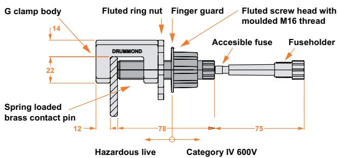
Disconnect 4mm plug before unscrewing fuseholder. Tighten fuseholder only finger tight. Ensure that the fuse (6.35 x 32mm) is correctly matched to application.
