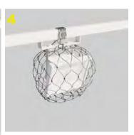
Tighten the stainless-steel lanyard and attach end to a secondary attachment point (to a sound body or structure).
