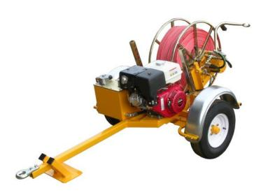
The CBS 680 Bulldog winch has been designed to provide a compact, transportable unit for overhead line stringing work. The self-contained winch is powered by an 11hp petrol engine and the precise control required is provided by the hydraulic circuit.
