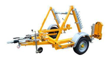
The C-751 Drum Trailer comes in three versions, and provides a compact and secure method of drum transportation. Manufactured in strong steel sections, it incorporates manually operated hydraulic lifting of drums.
