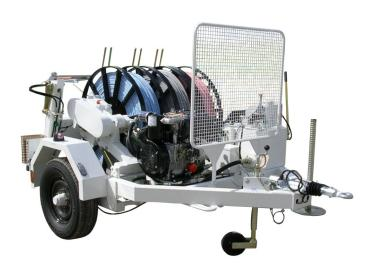
Designed to give reliable, flexible winching system to meet all 11/33kV work, together with some 66kV and 132kV maintenance requirements, the system employs a range of drums to suit particular applications.
