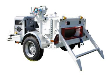
Hydraulic winch designed to provide reliable and safe lifting operations for tower and mast erection for the electricity or telecommunications industries. Winching is controlled via a proportional hydraulic valve giving the operator precise control over the load when needed or high speed if necessary.
