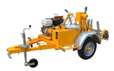
The CBS 821 Universal Winch offers the constant pulling tension of a double capstan drive and the flexibility of a direct drive drum in one machine.
