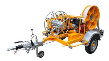
The C-1045 winch has been designed to meet the requirements of installing telecommunication cables, employing an 813mm diameter single capstan to impact a controlled force to the pulling rope or cable.
