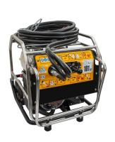
This unit is powered by air-cooled, 8hp petrol driven engine, delivering 20 litres/min at a working pressure of 138 bar from the hydraulic circuit. The circuit is protected with return line and filters. CE suction approved.
