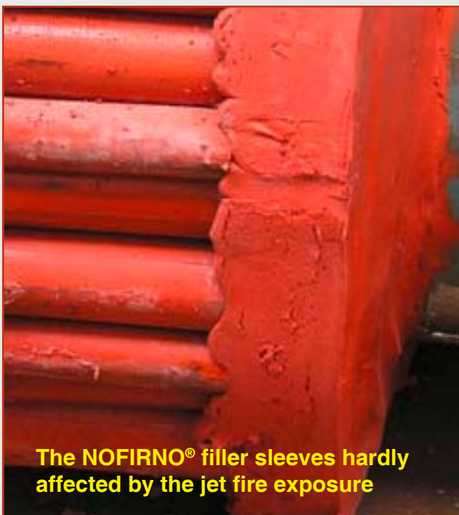
The NOFIRNO ® filler sleeves hardly affected by the jet fire exposure
