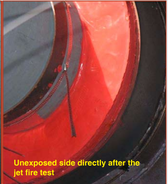
RISE ® /NOFIRNO ® exposed to a one hour Jet Fire Test
