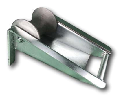
The MR1 manhole cable roller leads the cable from the drum into the jointbox/manhole or the winch bond out of the manhole. The roller has 2 hooks for location on the manhole edge
