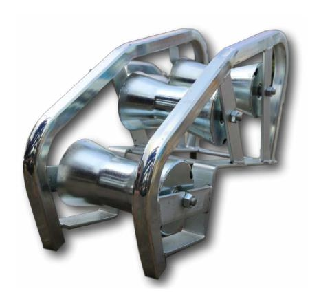
The MR4 manhole cable roller leads the cable from the drum into the jointbox/manhole or the winch bond out of the manhole. The cable roller is suitable for cables of up to 130mm
