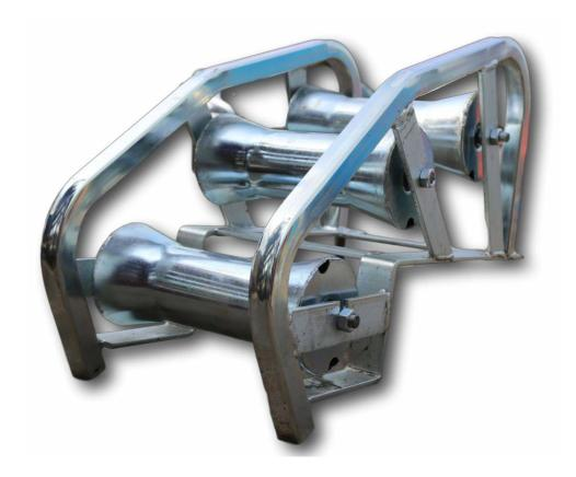
The MR6 manhole cable roller leads the cable from the drum into the jointbox/manhole or the winch bond out of the manhole. The cable roller is suitable for cables of up to 210mm
