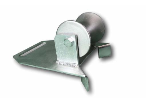
The MR2 manhole cable roller leads the cable from the drum into the jointbox/manhole or the winch bond out of the manhole. The roller has 2 angled hooks for location on the manhole edge or on a 90 degree corner
