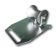
The MR3 manhole cable roller leads the cable from the drum into the jointbox/manhole or the winch bond out of the manhole. The roller has 2 angled hooks for location on the manhole edge or on a 90 degree corner. The unit is similar to the MR2 but the roller section swivels to suit the direction of the pull
