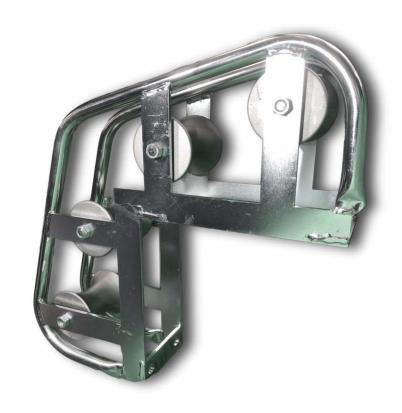
The MR5 manhole cable roller leads the cable from the drum into the jointbox/manhole, onto cable trays or out of the manhole. The roller is suitable for cables up to 90mm diameter. This can also be used on its side as a corner roller
