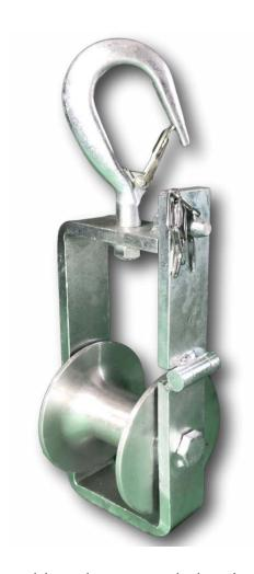
The HR2 hanging roller enables cable to be suspended and winched into position prior to fixing on to tray or cable racking. Fitted with a handy safety hook, the HR2 is quick and easy to install without the need for tools or shackles and is fitted with an aluminium deep diablo roller for effective cable management. The cable roller is suitable for cables up to 75mm diameter with a weight capacity of 100Kg
