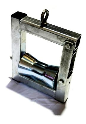
The HR1 hanging roller enables cable to be suspended and winched into position prior to fixing on to tray or cable racking. The cable roller is suitable for cables up to 120mm diameter with a weight capacity of 75Kg
