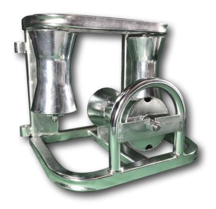
The BR3 is a heavy duty triple corner cable roller for use in most cable laying applications and for cables up to 130mm. These can be used singularly or linked together using link pins (LP1) to form a full bend. All of the bend roller range have the same link points to facilitate various bend/roller configurations
