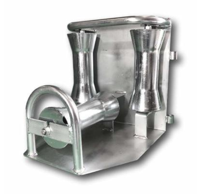
The BR6 is a heavy duty triple corner cable roller for use in most cable laying applications and for cables up to 210mm. These can be used singularly or linked together using link pins (LP1) to form a full bend. All of the bend roller range have the same link points to facilitate various bend/roller configurations
