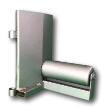
The BR1 is a medium duty corner cable roller for use in most cable laying applications. These can be used singularly or linked together using link pins (LP1) to form a full bend. All of the bend roller range have the same link points to facilitate various bend/roller configurations. The bottom roller passes through the skid plate to ensure the pulling bond or cable cannot get trapped or damaged
