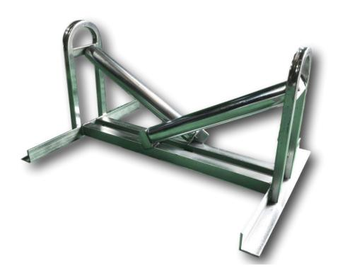
The V style cable roller leads the cable from the drum into the trench, the design is such that cable is centralised prior to it being fed into the trench. This roller also doubles up as a heavy duty straight line roller or pipe roller and can be positioned in the trench itself. Any width or capacity of V roller can be made on request
