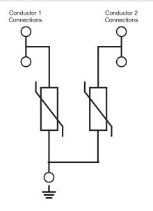
\*N.B. Device is not polar - Input and output connections can be reversed
