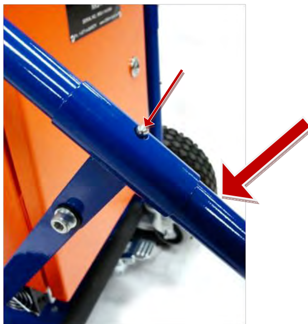
Figure J-5: Unlocking the Transport Assist leg for stowing
