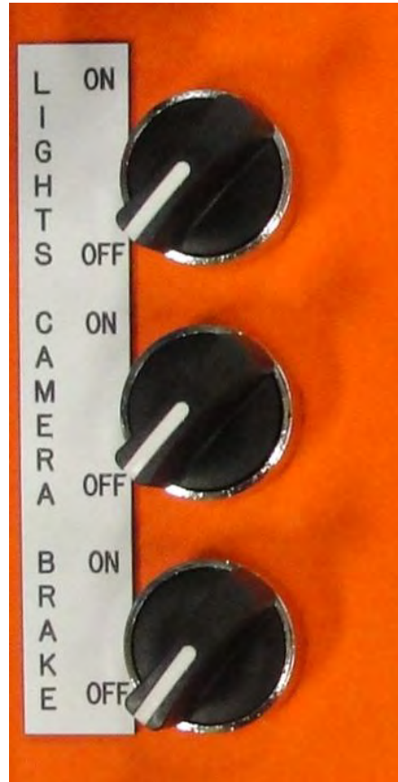
Figure F-2: Standard switch layout showing “CAMERA” switch in the “OFF” position
